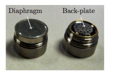
This photo represents two electrostatic microphone capsules. Here, the membrane acts as the mobile electrode of the transducer (visible on the left capsule). The perforated rear electrode is visible on the right capsule due to the removal of the membrane. This electrode is the transducers immobile electrode
