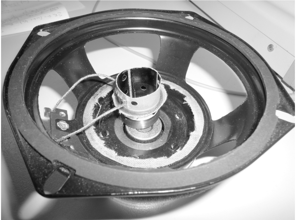
Coil removed from the motor
